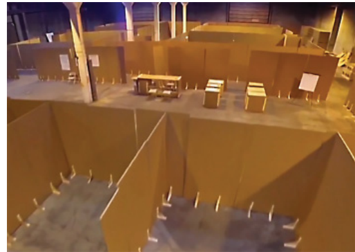
A full-scale mockup of a hospital facility, constructed from PCA's Hexacomb® material, fills a warehouse space.
